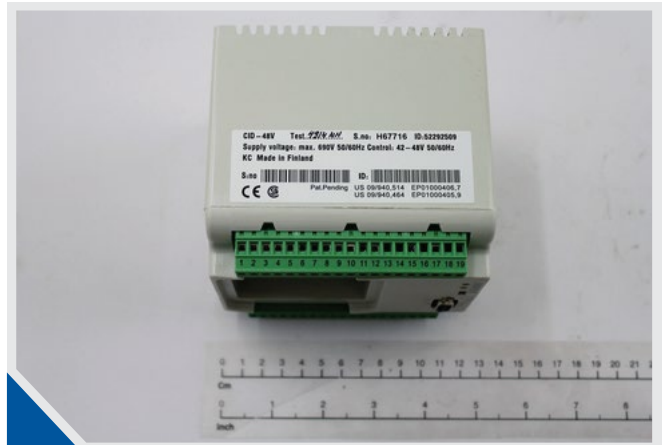
Condition monitoring unit
